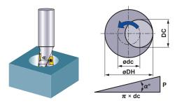
How to calculate the theoretical center of the cutter path.
