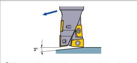
• When machining steel the recommended ramping angle is 3°. If a ramping angle larger than 3° is used, then the chips may not be broken effectively resulting in chips wrapping around the tool.
