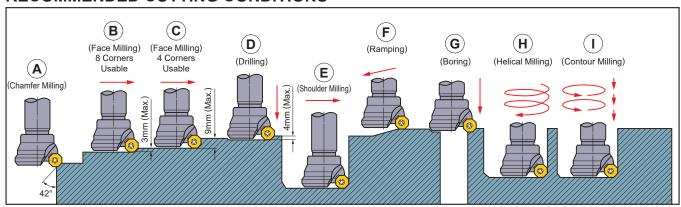
This list of recommended cutting conditions is for cutters with diameter ≤ \$\phi 80\$. For cutters with diameter greater than \$\phi 80\$ increase cutting speed by around 10%. Above sizes are for OEMX1705.......
